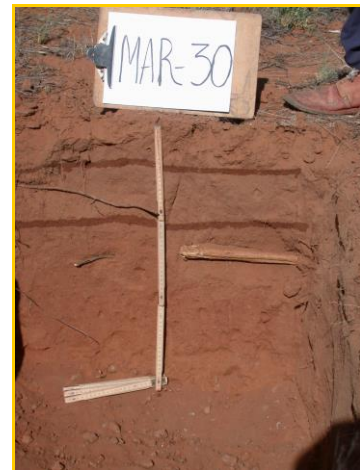
This soil type have been blown in from neighbouring region and deposited on the irregular quartzitic fragments.
