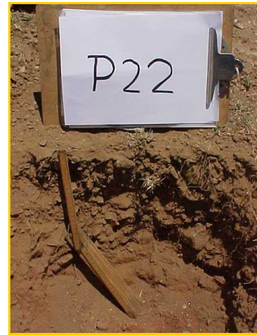
Skeletal Regosols is the dominant soil within this unit. The soils are shallow to moderately deep with many to abundant rock fragment in the profile.
