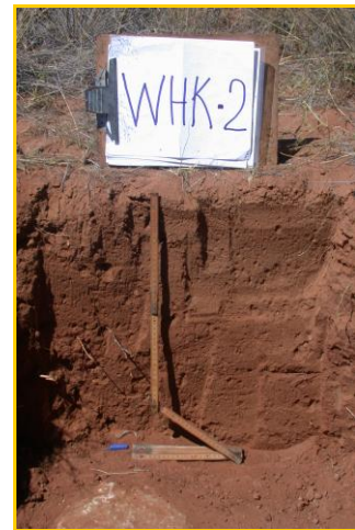
Moderately deep, aridic ferralic Arenosols underlying by hard gneiss rock that restrict the down movement of plant roots and water.
