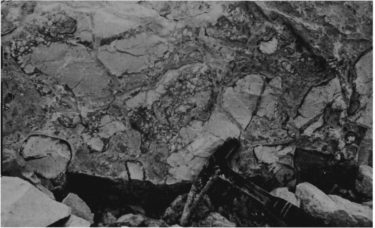
Figure 34 Brecciated, very hard hardpan calcrete exposed by blasting for road quarry near Tsumeb, South West Africa.
