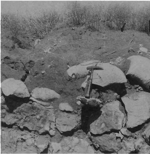
Figure 35 Calcrete hardpans weathering to boulders exposed in quarry near Pienaars River, Transvaal. Note rounded tops of boulders in upper boulder horizon.
