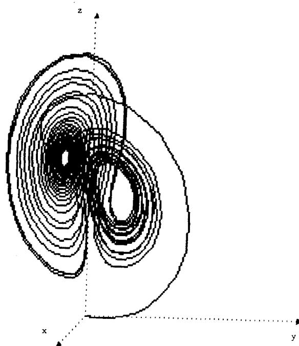
Figure 4: Plot of a curve approaching the Lorenz attractor as obtained by a student using the modified Euler method with x(0) = 0.00001, y(0) = 0.00001 and z(0) = 0.00001 .
